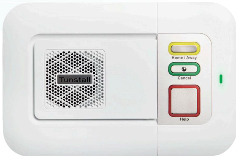
It works from your electricity supply connected by a plug to one of your sockets. It also has a backup battery in it. The Hub is generally located in your living room. It has an in built SIM card which uses 5G technology to transmit a signal.
